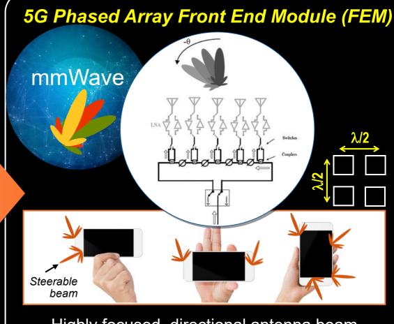
Highly focused, directional antenna beam Secure & immune to interference High data rates and user density/capacity
