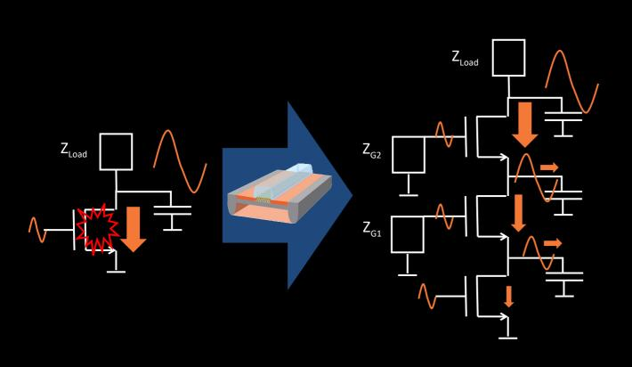
Electrically Isolated Body in FD-SOI Allows Transistor Stacking for Large Signal in PA and Switch
