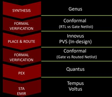
Tape-out proven Flow **GF** Digital Design Reference Flow
