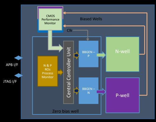
Closed-loop Control to Provide Adaptive Body Bias
